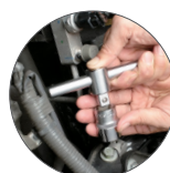
Sliding T-handle with quick release
