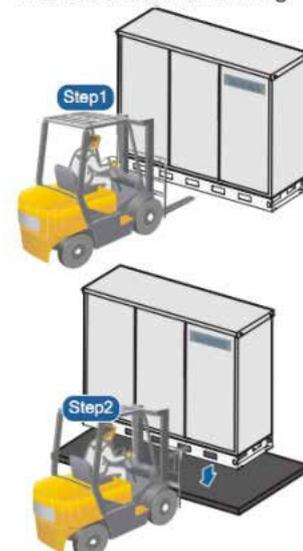
(2) One unit cabinet shall be completely installed and transported before leaving the factory. After arriving at the construction site, first remove the outer packaging, then install the cabinet on the cement base with a lifting device, connect it with the anchor bolts, and finally lock it with nuts. The structure is shown in Fig. 2.
