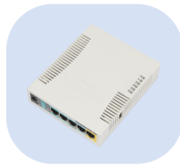
WIRELESS ACCESS POINT ROUTER (RB951UI-2HND)
